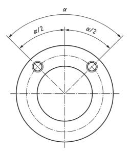
Figure 3 — Positions of the holes for the studs/bolts
